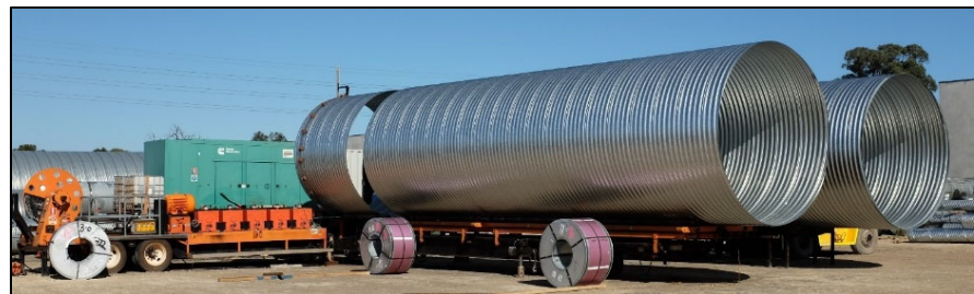
Roundel Stilcor Mobile CSP Pipe Mill
