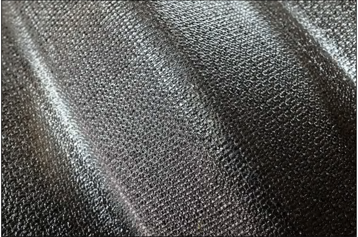
HPL PE-coated steel - close up
